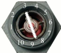
Using the supplied plastic key, fit it into the slots as shown, Turn clockwise to increase, and anti clockwise to decrease the quantity of water required. For washing machines set to position 8 and dishwashers to position 4
