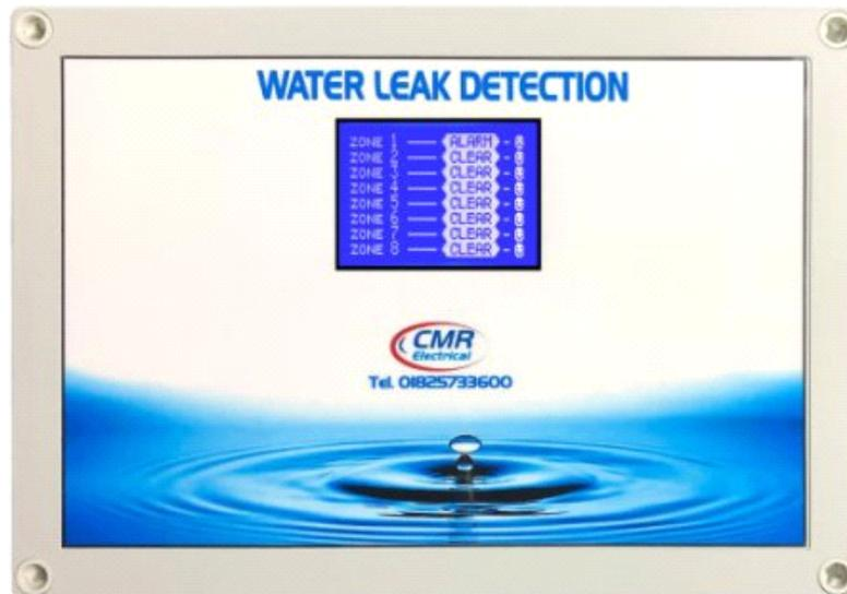
The LD8-2 range has been designed to monitor eight independent zones in critical areas for water leaks via liner detection cables or spot sensors. Any number of spot sensors or a maximum of 50 metres of liner water detection cable can be connected to each zone.
