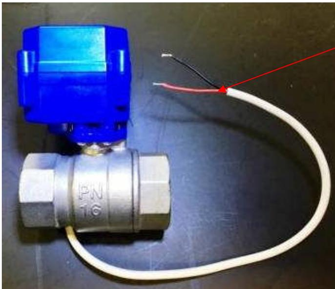
The 230VAC supply to the valves is generated from within the alarm unit. 15 to 25mm valves are supplied with a red and black cable whilst larger valves are red and green. For good practice connect live to the red wire and neutral to the black or green wire.
