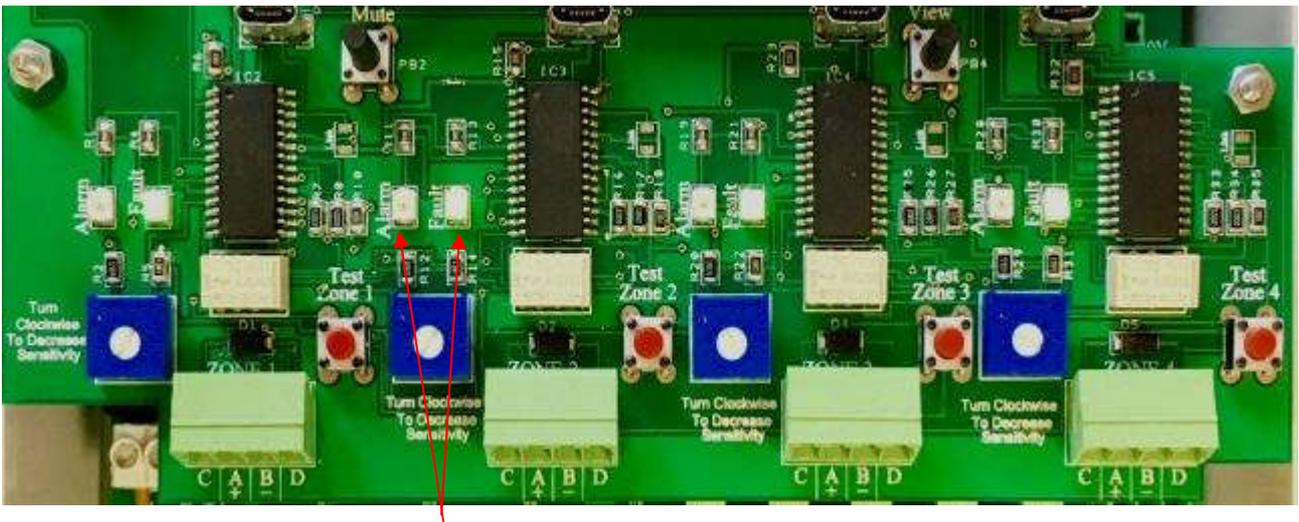
To help with fault diagnoses individual “Alarm” and “Fault” lamps are provided so show the status of each zone.
