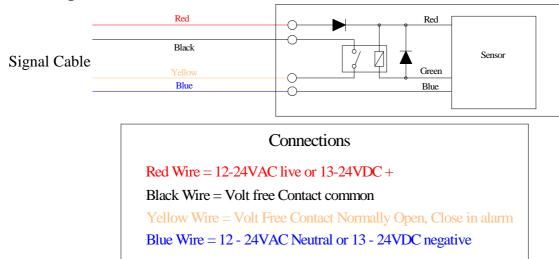
The signal cable should be terminated between the sensor and the main Alarm/BMS in the following manner.
