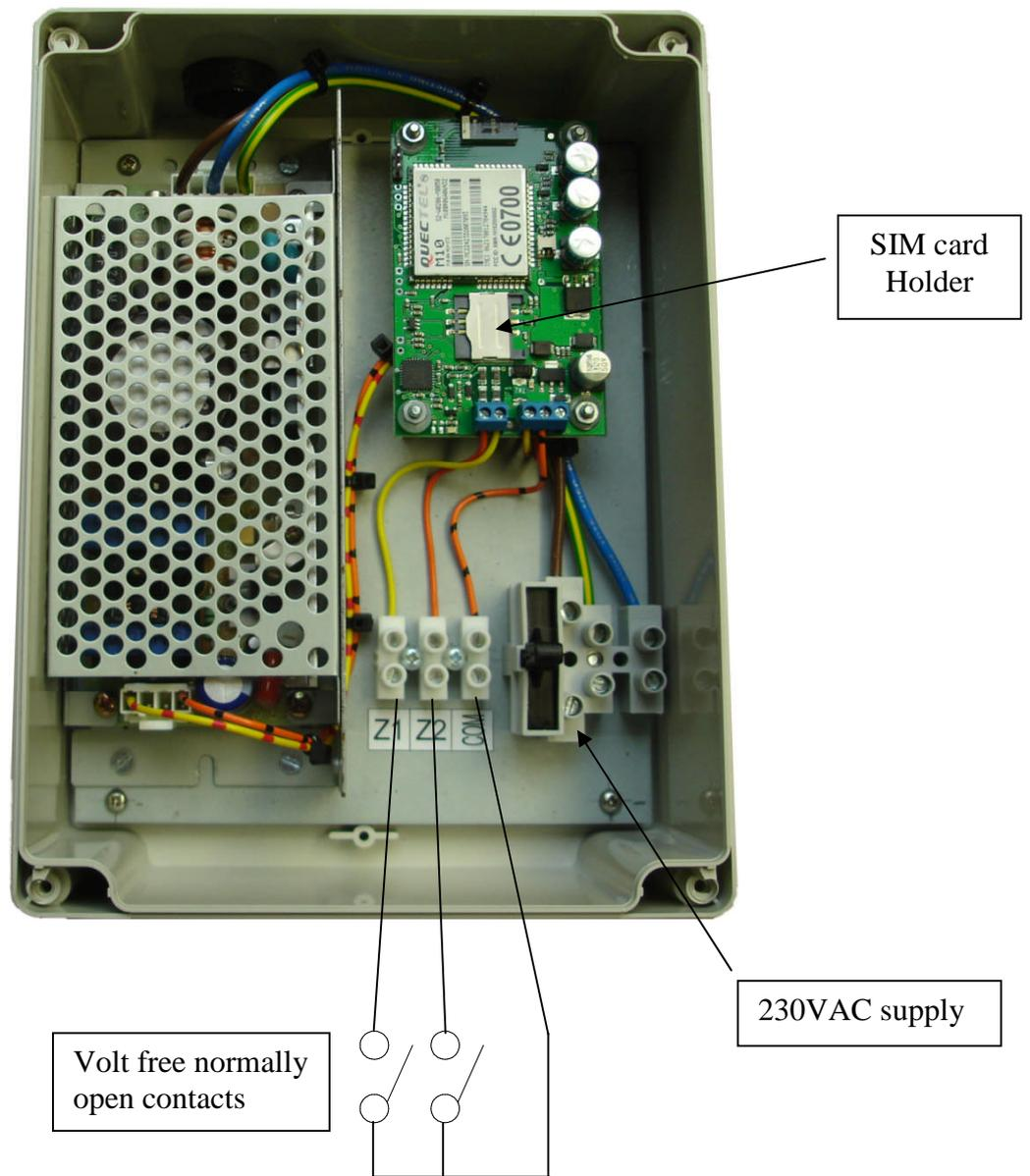
Close contact between “Com” and “Z1” for zone 1 alarm, close contact between “Com” and “Z2” for zone 2 alarm.
