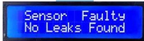
The temperature sensor has become disconnected or faulty
