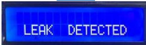
Water leak Alarm; this statement will flash until the "Mute" button is pressed
